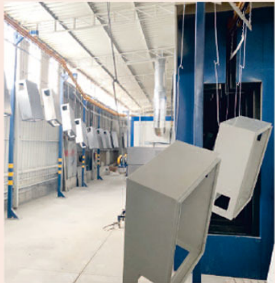
Tam otomatik boyahane hattı (Fully automated painting line)
